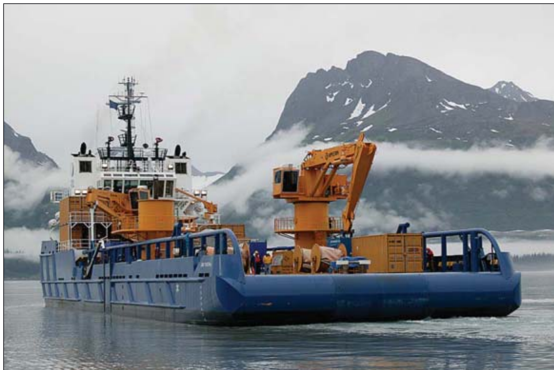
The Chouest Nanuq is a new, ice-strengthened barge built in Louisiana for the Beaufort Sea work (Fig. 5; photo from Shell Alaska).
