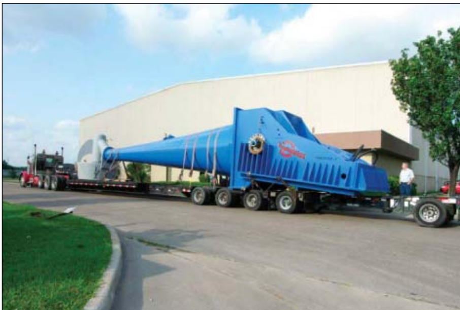
Each of the two new thrusters built by ThrustMaster of Texas Inc. for the Kulluk weighs about 62 tonnes (Fig. 4; photo from Thrust Master).
